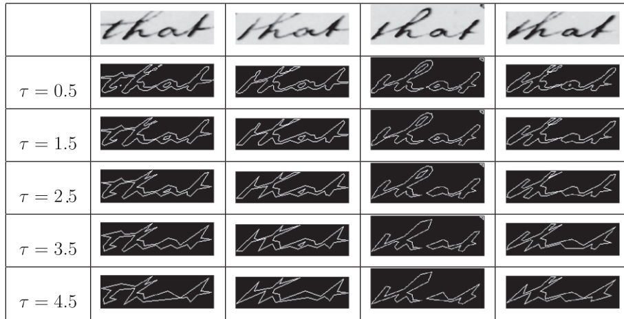
Fig. 4. Representation of the lines fitted into the points of the contour segments on our instances of the word that, for \tau values 0.5, 1.5, 2.5, 3.5, and 4.5, respectively. Note that, different instances of a word may have different number of contour segments, and different number of extracted lines due to the writing style. There may be noise inside the segmented word images, or parts of the word may be cut due to wrong segmentation. Most of these problems are handled by extraction of lines in different levels of details.
