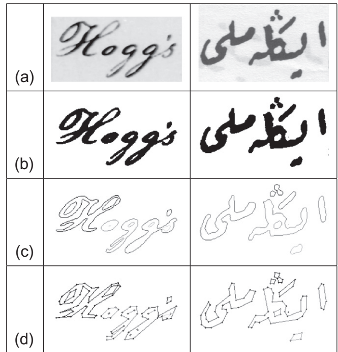
Fig. 3. Line extraction process on sample words. (a) Original gray-scale word images. (b) Binarized forms of the original gray-scale word images. (c) Contour segments extracted from the binarized forms of the images. (d) Approximated lines on the points of contour segments ( \tau = 3.0 ). Note that, a single word may consist of multiple the contour segments, and the holes inside a character usually correspond to separate contour segments.
