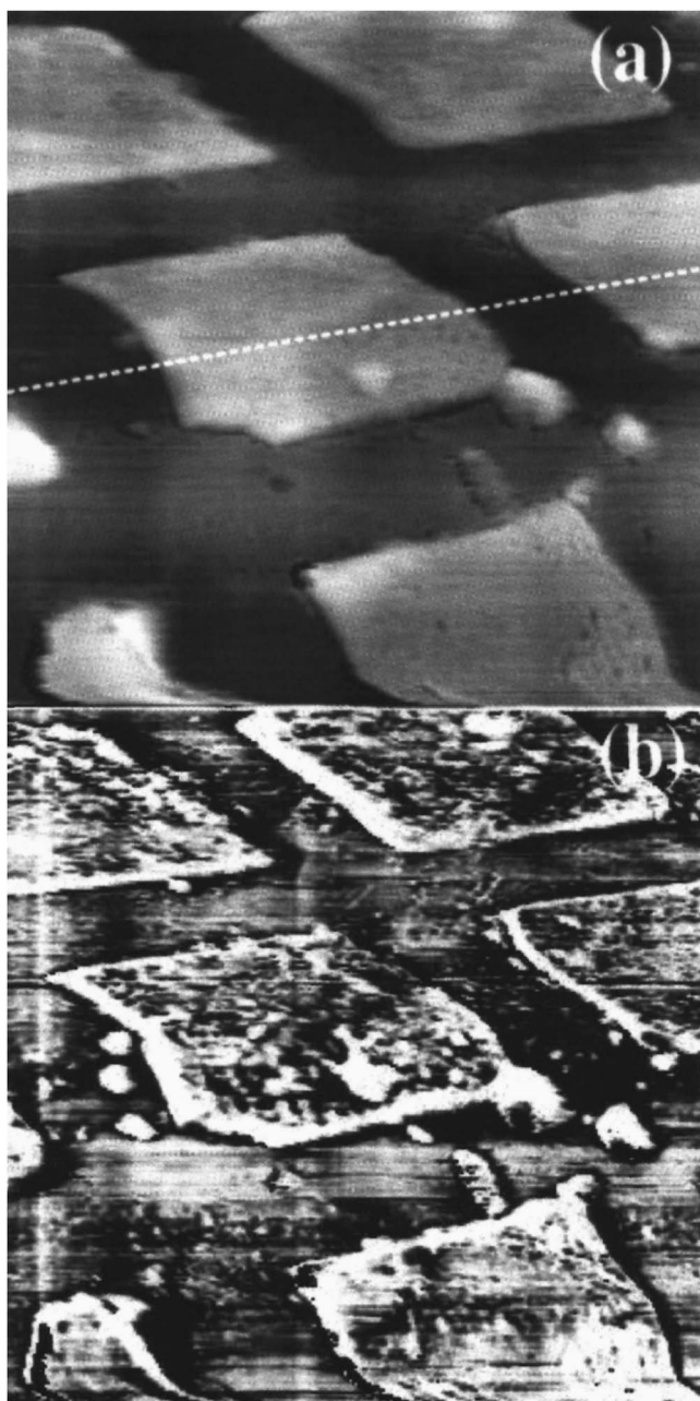
FIG. 4. (a) Topography and (b) third-harmonic amplitude. Scan size is 15 \times 15 \mu\text{m} . Grayscale is 320 nm in (a) and 0.91 nm in (b).
