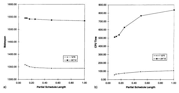
Fig. 5. Interactions between makespan and CPU time and partial schedule length (uniform case). (a) Frequency level of 14. Makespan vs partial schedule length. (b) Frequency level of 14. CPU time vs partial schedule length.
