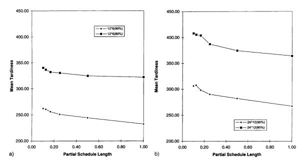
Fig. 6. Mean tardiness vs partial schedule length in 90% and 80% efficiency levels, uniform case. (a) Frequency level of 14, 12 jobs and 6 machines. Mean tardiness vs partial schedule length. (b) Frequency level of 14, 24 jobs and 12 machines. Mean tardiness vs partial schedule length.
