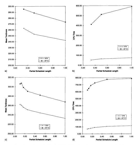
Fig. 3. Mean tardiness and CPU time as a function of partial schedule lengths (uniform case). (a) Frequency level of 4. Mean tardiness vs partial schedule length. (b) Frequency level of 4. CPU time vs partial schedule length. (c) Frequency level of 14. Mean tardiness vs partial schedule length. (d) Frequency level of 14. CPU time vs partial schedule length.
