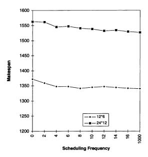
Fig. 2. Interactions between scheduling frequency and makespan values.
