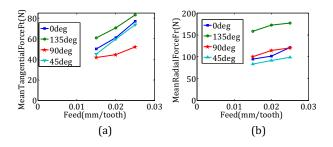
Fig. 5. (a) Mean tangential and (b) radial forces as functions of feed per tooth.
