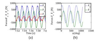
**Fig. 8.** Validation of slot milling force predictions for six tooth milling tool: N = 4000 rpm,  $f_r = 1250 \text{ mm/min}$ , 100% radial immersion,  $a_p = 10 \text{ mm}$ . (a) Measurement and (b) prediction.
