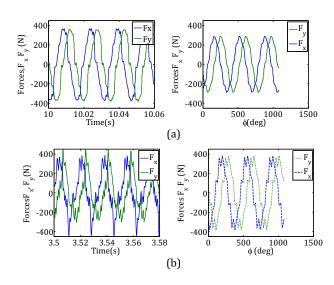
**Fig. 7.** Comparison of experimental data (left) and model predictions (right) for two different milling cases: (a) N=4000 rpm,  $f_r=254$  mm/min, 100% radial immersion,  $a_p=10$  mm and (b) N=3500 rpm,  $f_r=750$  mm/min, 50% radial immersion downmilling,  $a_p=10$  mm.
