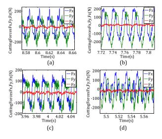
**Fig. 4.** Milling force measurements during slot milling. (a)  $0^{\circ}$ , (b)  $135^{\circ}$ , (c)  $90^{\circ}$ , and (d)  $45^{\circ}$ .
