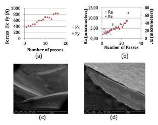
**Fig. 9.** (a) Milling force and (b) surface roughness variation due to tool wear as a function of cutting distance (N = 4000 rpm,  $f_r = 254 \text{ mm/min}$ , 100% radial immersion,  $a_p = 10 \text{ mm}$ ). (c and d) SEM images of fractured diamond coating.
