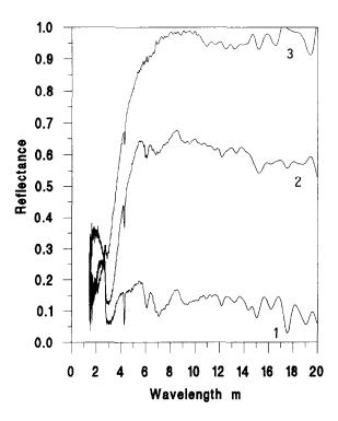
Fig 1: Spectra of the pigmented aluminium oxide at different conditions, 1 and 2 pigmented by NiSO<sub>4</sub>, 3 pigmented by Ni(CH<sub>3</sub>COO)<sub>2</sub>
