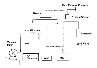
**Fig. 1.** Diagrammatic representation of glow discharge plasma.
