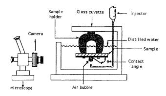
Fig. 2. Schematic view of entrapped air-bubble technique.
