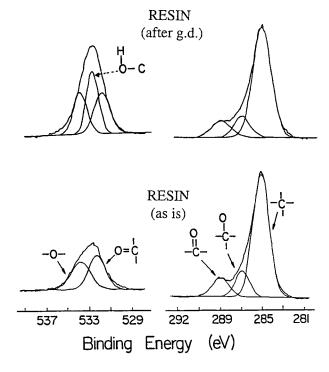
**Fig. 3.** O1s and C1s XPS of untreated (control) and glow discharge—treated resin at 90-degree take-off angles. Enhanced O1s signal is assigned to –COH.
