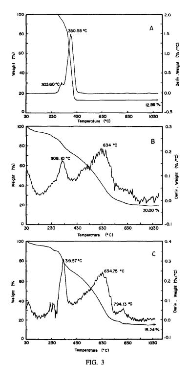
Thermogravimetric analysis of (A) PMMA-co-PEMA-0.7, (B) PPy/PMMA-co-PEMA-0.7 ( $BF_4^-$  doped), and (C) PPy/PMMA-co-PEMA-0.7 ( $ClO_4^-$  doped).
