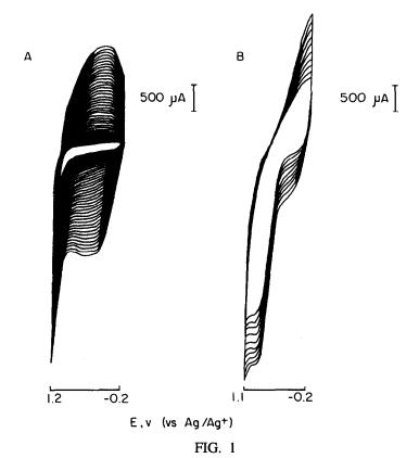
Cyclic voltammogram of (A) PPy/PMMA-co-PEMA-0.7 in TBAFB-acetonitrile and (B) pyrrole on a PMMA-co-PEMA-0.7 coated electrode in  $NaClO_4$ -water medium.
