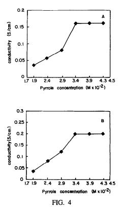
Conductivity versus feed pyrrole for (A) PPy/PMMA-PEMA-0.7 ( $BF_4^-$  doped) and (B) PPy/PMMA-PEMA-0.7 ( $CIO_4^-$  doped).
