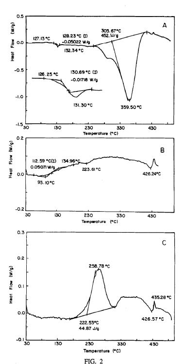
DSC thermogram of (A) PMMA-co-PEMA-0.7, (B) PPy/PMMA-co-PEMA-0.7 ( $BF_4^-$  doped), and (C) PPy/PMMA-co-PEMA-0.7 ( $CIO_4^-$  doped).
