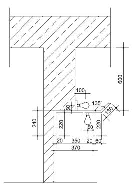
Fig. 7. Lamp installations of wall washing and cove lighting.
