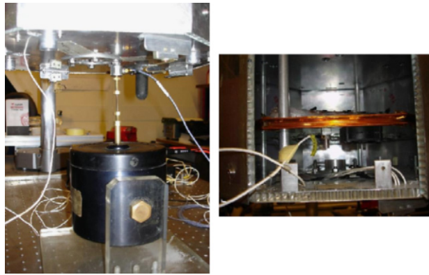
Fig. 5. On the left: electro-dynamic exciter acting on the bottom panel of the satellite. On the right: inner view of the satellite structure.
