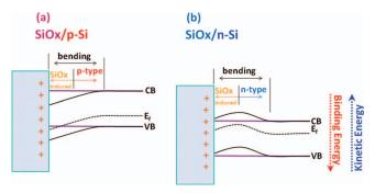
FIG. 5. Schematic representation of the variations in the band-bending at the oxide-Si interface for (a) p- and (b) n-Si.
