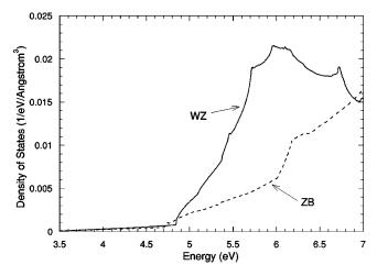
FIG. 2. Density of states per spin, per volume of the ZB (dashed) and WZ (solid) phases of GaN for the lowest conduction-band energies. The zero level of the energy is set to valence-band maximum.
