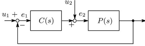
Fig. 1. Closed-loop system.
