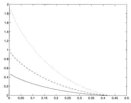
Fig. 2. Curves of  $E(D, \rho)$  versus D for a binary source with letter probabilities p(0) = 1 - p(1) = 0.4, and the Hamming distortion measure. The solid line corresponds to  $\rho = 0.5$ , the dashed line to  $\rho = 1$ , and the dotted line to  $\rho = 2$ .
