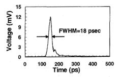
Fig. 3. Pulse response of RCE Schottky photodiode.
