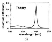
Fig. 2. (a) Measured photoresponse of RCE photodiode and (b) simulated photoresponse of the same structure.
