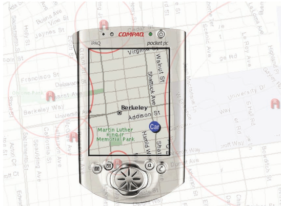
Figure 4. The Halo approach displays arcs at the detailed view's borders. The ring's radius is proportional to the distance.
