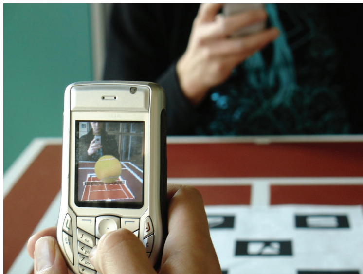
Figure 6. In AR Tennis, the camera tracks markers on the table and the other player's camera. The players attempt to bounce the ball back and forth in a virtual tennis court.
