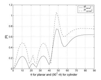
Fig. 7. Magnitude of the reflection coefficient |R| vs. scan angle in the E plane for the center element of an array of  $11 \times 11$  printed dipoles on both cylindrical and planar geometries. Cylinder same as in Fig. 5.
