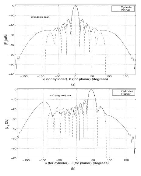
Fig. 9. Far-field patterns of printed dipole arrays on both the cylinder and planar substrates. All arrays are periodic with  $0.5\lambda_0$  in all directions and (a) 9 × 9 printed dipole arrays are phased to radiate along the broadside direction, (b)  $11 \times 11$  printed dipole arrays are phased to radiate a beam maximum in the direction of 45°. Cylinder same as in Fig. 5.
