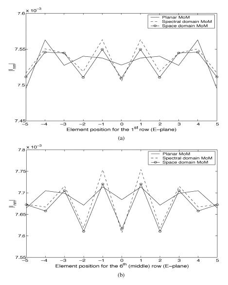
Fig. 5. Comparison of the magnitude of the induced current  $|I_{nm}|$  obtained via cylindrical spatial, cylindrical spectral and planar MoM for the (a) first row (E plane) (n = -5 : 5 and m = -5); (b) middle (6th) row (E plane) (n = -5 : 5 and m = 0) of a 11 × 11 printed dipole array. Cylinder parameters:  $a = 3\lambda_0$ ,  $t_h = 0.06\lambda_0$  and  $\epsilon_r = 3.25$ .
