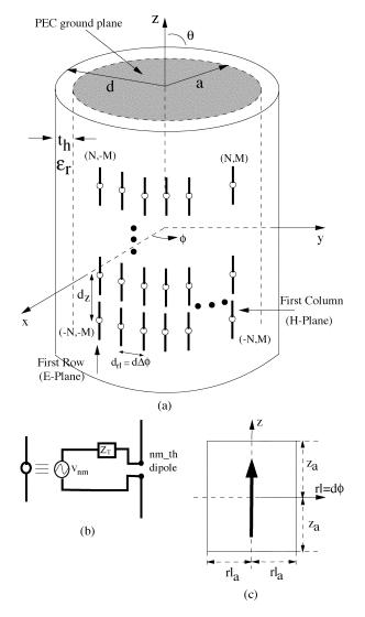
Fig. 1. (a) Geometry of a periodic array of  $(2N + 1) \times (2M + 1)$  printed dipoles on a dielectric coated, electrically large circular cylinder. (b) Dipole connected to an infinitesimal generator with a voltage  $V_{nm}$  and a terminating impedance  $Z_T$ . (c) Representation of each dipole for the Method of Moments (MoM) calculations.
