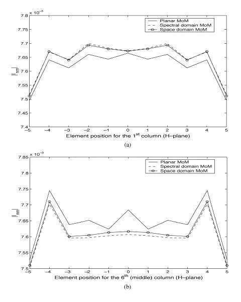
Fig. 6. Comparison of the magnitude of the induced current  $|I_{nm}|$  obtained via cylindrical spatial, cylindrical spectral and planar MoM for the (a) first column (H plane) (m = -5 : 5 and n = -5); (b) middle (6th) column (H plane) (m = -5 : 5 and n = 0) of a 11 × 11 printed dipole array. Cylinder same as in Fig. 5.
