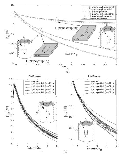
Fig. 4. Magnitude of the mutual coupling  $Z_{12}$  versus separation s between two identical printed dipole modes along the E and H planes for a coated cylinder with  $\epsilon_r = 3.25$  and  $t_h = 0.06\lambda_0$ . The dimension of each dipole is  $(L, W) = (0.39\lambda_0, 0.01\lambda_0)$ . The radii of the cylinders are (a)  $a = 3\lambda_0$ , (b)  $a = 2\lambda_0$ ,  $a = 3\lambda_0$ ,  $a = 4\lambda_0$ ,  $a = 5\lambda_0$ , respectively.
