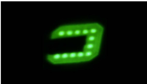
Fig. 18. (Color online) An image of the LED array on the object plane: the object is first imaged onto this plane by a projector lens to control both the depth and the size of the object.
