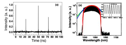
Fig. 6. (a) 5 GHz-oscilloscope trace of a pair of bound pulses and a single pulse. (b) Optical spectrum of co-emission of a pair of bound pulses and a single pulse. The open circles are theoretical fit for a parabolic pulse shape. The closed squares (triangles) are for Gaussian ( $sech^2$ ) fit and the inset shows a magnified portion of the optical spectrum on a linear scale.
