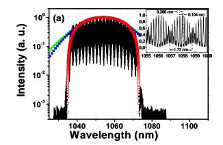
Fig. 4. Optical spectrum of the triplet featuring different separations. The spectrum is fit with parabolic (open circles), Gaussian (closed squares), and sech<sup>2</sup> (closed triangles) pulse shapes. The inset shows a magnified portion of the optical spectrum on linear scale.
