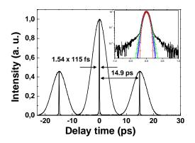
Fig. 3. Autocorrelation trace of the dechirped (solid line) and chirped (dashed line) twin bound state pulses. Inset shows the central peak of the autocorrelation trace after extracavity dechirping on a logarithmic scale. The theoretical fits with parabolic (open circles), Gaussian (closed square curves) and sech<sup>2</sup> (closed triangle curves) pulse shapes are also shown on the inset. Pulse duration assuming a sech<sup>2</sup> shape is 115 fs.
