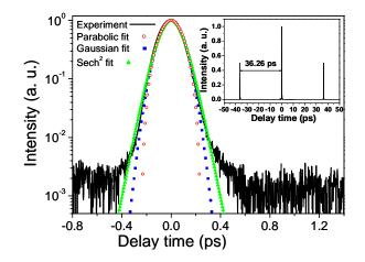
Fig. 7. Central peak of the autocorrelation trace after extra-cavity compression in the case of co-emission of a pair of bounded pulses and a single pulse. The inset shows the complete autocorrelation trace. Pulse duration assuming a sech<sup>2</sup> shape is 100 fs.
