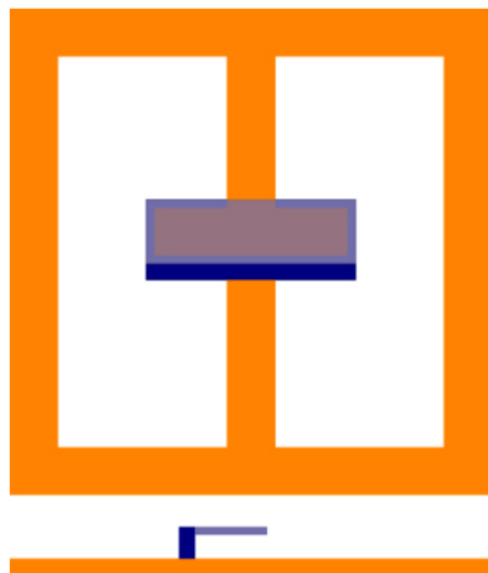
Fig. 1b. The structure and the transfer characteristics of an eSRR modified to incorporate a parallel plate capacitor. For the device simulated the sides are 120\ \mu\text{m} , the arms are 10\ \mu\text{m} , the height of the top plate from the bottom plate is 3\ \mu\text{m} , and the bottom plate is 60 \times 4\ \mu\text{m} square.
