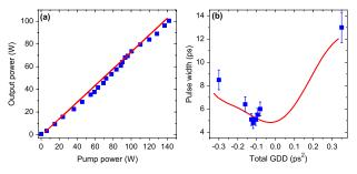
Fig. 3. (Color online) (a) Measured (squares) and simulated (solid line) output power versus pump power; (b) measured (squares) and simulated (solid line) pulsewidth at 100 W power versus total GDD of the system.
