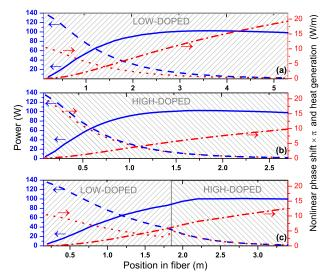
Fig. 2. (Color online) Simulated evolution of signal (solid curve) and pump (dashed curve) power, nonlinear phase shift (dot-dashed curve) and heat generation per unit length (dotted curve) along (a) low-doped, (b) high-doped, and (c) low- and high-doped, hybrid gain fibers.
