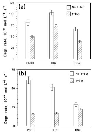
**Figure 2.** Photocatalytic degradation rates of PhOH, HBz and HSal (initial concentration 0.25 mmol  $L^{-1}$ ), with and without addition of 10 mmol  $L^{-1}$  t-butanol, in the presence of 0.2 g  $L^{-1}$  TiO<sub>2</sub> P25 (a) and W (b) at pH 3, adjusted with HClO<sub>4</sub>. The error bars represent  $\sigma$ -level uncertainties.
