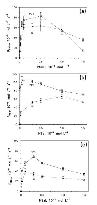
**Figure 3.** Initial photocatalytic degradation rates of PhOH (a), HBz (b) and HSal (c) as a function of substrate concentration, in the presence of  $0.2 \text{ g L}^{-1} \text{ TiO}_2$  (P25 or W) at pH 3, adjusted with HClO<sub>4</sub>. The error bars represent  $\sigma$ -level uncertainties.
