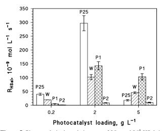
**Figure 5.** Photocatalytic degradation rate of 25  $\mu$ mol L<sup>-1</sup> HSal, in the presence of the four tested photocatalysts (P25, W, P1, P2) at different loading values. The pH of the suspensions was 3, adjusted with HClO<sub>4</sub>. The error bars represent  $\sigma$ -level uncertainties.
