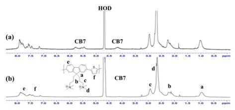
Fig. 2 <sup>1</sup>H-NMR (400 MHz, 298 K, D<sub>2</sub>O) spectra of (a) P2CB7 (b) P2.
