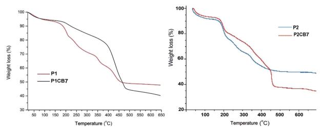
Fig. 3 TGA curves of polymers P1, P2 and polyrotaxanes P1CB7, P2CB7 under N<sub>2</sub> at 10 °C min<sup>-1</sup>.
