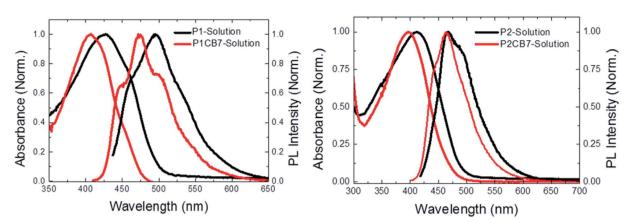
Fig. 4 UV-vis absorption and emission spectra of P1, P2, P1CB7 and P2CB7 in aqueous media
