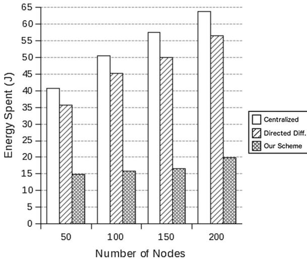
Fig. 8 Average energy consumption by sensor nodes
