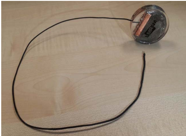
FIG. 2. Picture of the TSI device. The electronic circuit and the battery are inside a 50-mm-diameter titanium case with a 2-mm-thick polydimethylsiloxane coating. A 60-cm-long lead with a diameter of 2.3mm was connected to the case. The electrode at the tip of the lead has a 6 mm 2 surface area.
