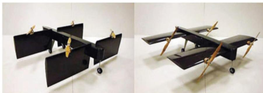
**FIGURE 1** Quad tilt-wing unmanned aerial vehicle (Sabanci University Unmanned Aerial Vehicle) with 2 different wing-angle configurations. [Colour figure can be viewed at [wileyonlinelibrary.com](http://wileyonlinelibrary.com)]
