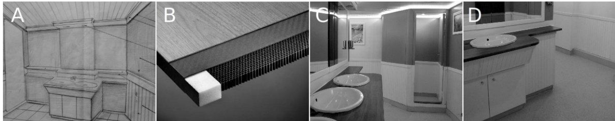
Figure 6a, b, c, d. Design proposal for renovation of restroom 1. An example of an interior panel made with Pre-Preg Carbon laminates on a Nomex sandwich and visible surface covered with a thin Teak veneer. Restrooms realization. Source: Siniša Prvanov.
