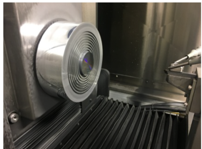
Fig. 1 Diamond turning experimental setup
