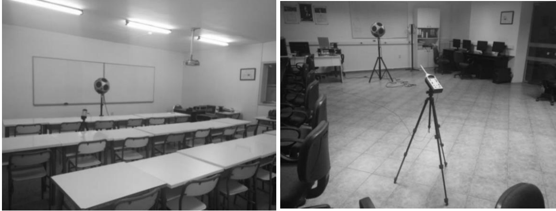
Figure 4: In-situ measurements of T30 and STI in unoccupied condition
