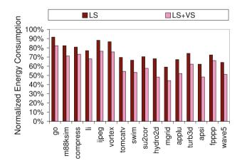
Fig. 2 Energy consumption results with the default simulation parameters. LS: link shutdown; LS + VS: link shutdown followed by voltage scaling
