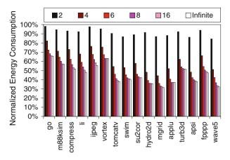
Fig. 3 Impact of the number of voltage/frequency levels. The last *bar*, for each benchmark, captures continuous scaling
