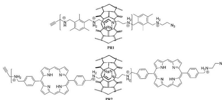
**Figure 5.** The structures of polyrotaxanes **PR1** and **PR2**. **PR1**, from monomers **7** and **8**, and **PR2**, from monomers **10** and **11**, were synthesized using CB6 as a macrocycle and catalyst. Chloride counterions have been omitted for clarity.
