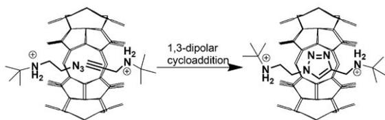
**Figure 3.** Synthesis of [2] rotaxane by CB6-catalyzed 1,3-dipolar cycloaddition.
