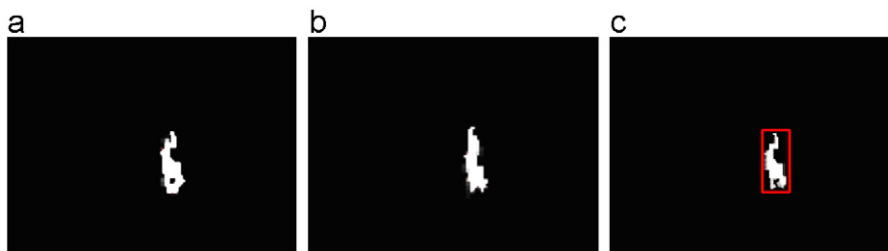
Fig. 10. Region overlap detection: (c) logical AND of (a) visual and (b) amplitude candidate flame regions.
