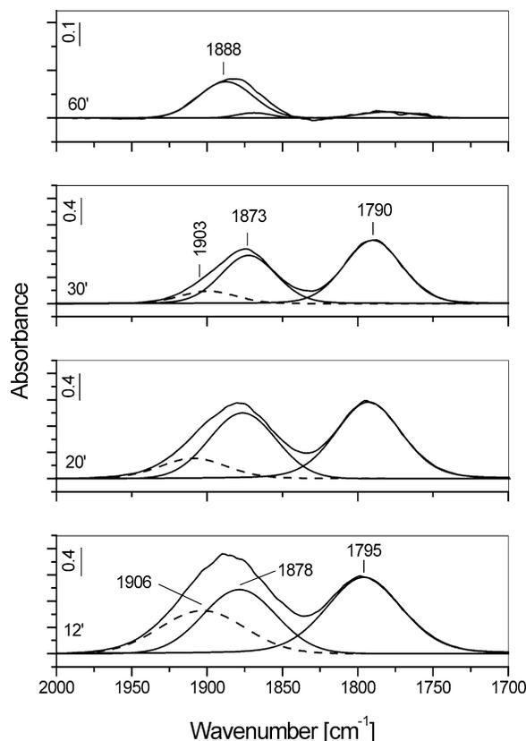
Fig. 11. Results of the curve-fitting procedure applied to the FT-IR spectra in the 2000–1700 cm<sup>-1</sup> region taken at various times of NO adsorption (1.07 kPa, room temperature) on the 5CoSZ sample.
