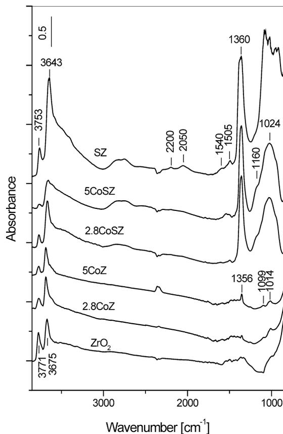
Fig. 2. FT-IR spectra of the activated catalysts and supports used.
