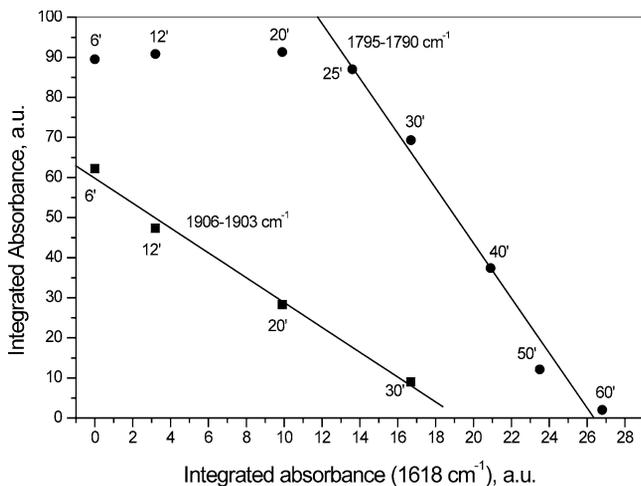
Fig. 10. Correlation between the integrated absorbances of the bands due to the  $\nu(\text{NO})$  and  $\nu_{\text{as}}(\text{NO})$  modes of the cobalt(III) mono- and cobalt(II) dinitrosyls and the integrated absorbance of the  $\delta(\text{H}_2\text{O})$  band at 1618 cm<sup>-1</sup> produced during NO adsorption (1.07 kPa, room temperature) at various times on sample 5CoSZ.
