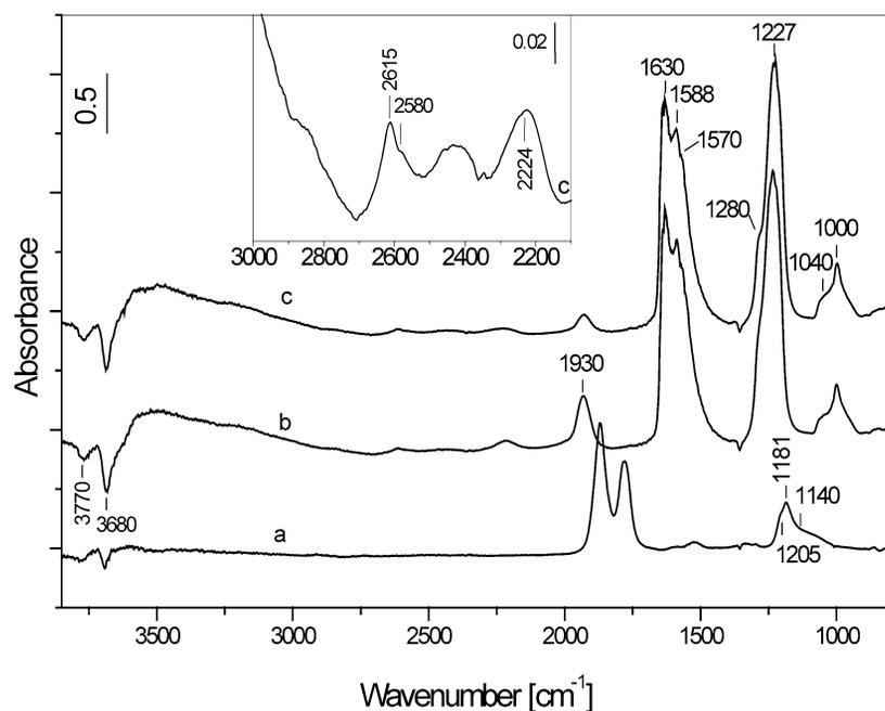
Fig. 7. FT-IR spectra of NO (0.67 kPa) (a) adsorbed on sample 5CoZ at room temperature for 5 min, (b) after subsequent introduction of  $\text{O}_2$  (0.67 kPa) for 30 min, and (c) after evacuation for 15 min at room temperature. The spectrum of the activated sample is used as a background reference.
