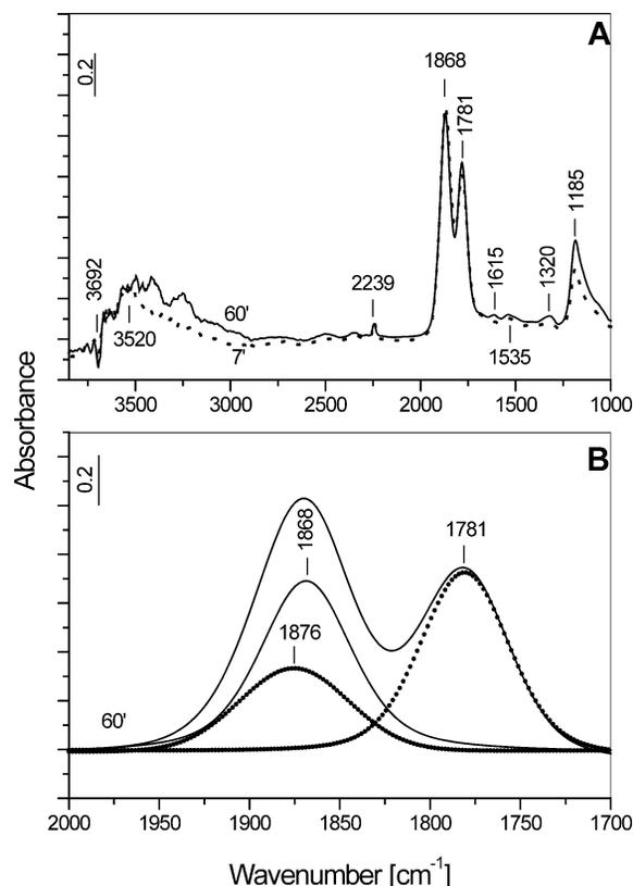
Fig. 3. (A) FT-IR spectra of NO ( $1.07\text{ kPa}$ ) adsorbed at room temperature on the 2.8CoZ catalyst for 7 and 60 min. The spectrum of the activated sample is used as a background reference. (B) Results of the curve-fitting procedure applied to the FT-IR spectrum in the  $2000$ – $1700\text{ cm}^{-1}$  region taken 60 min after the NO adsorption ( $1.07\text{ kPa}$ , room temperature) on the 2.8CoZ sample.
