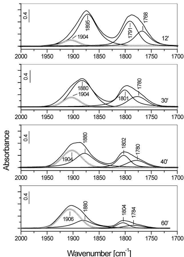
Fig. 5. Results of the curve-fitting procedure applied to the FT-IR spectra in the  $2000\text{--}1700\text{ cm}^{-1}$  region taken at various times of NO adsorption (1.07 kPa, room temperature) on the 5CoZ sample.
