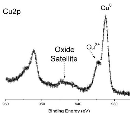
**Fig. 6** Cu2p region of the XPS spectrum of AgCu nanoalloys after storing for 75 days, showing an additional CuO<sub>x</sub> satellite structure.
