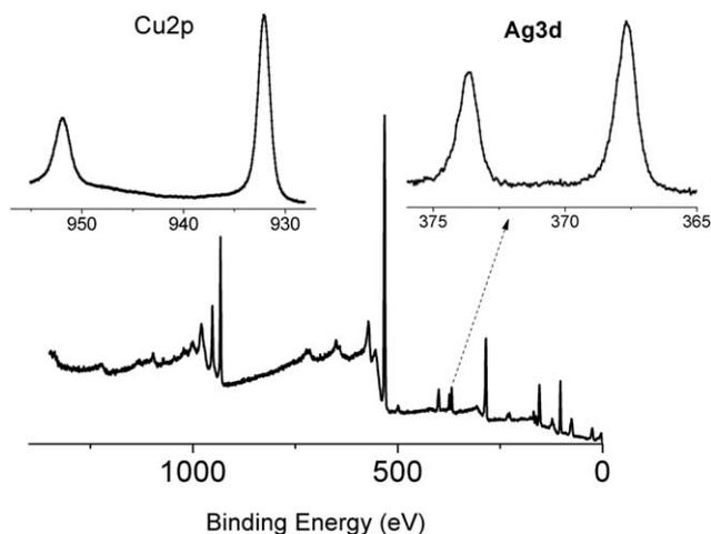
Fig. 3 XPS spectrum of AgCu alloy nanoparticles.
