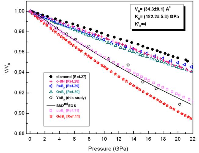
**Figure 6.** Volume compression of  $\text{YbB}_2$  as a function of pressure with a Birch–Murnaghan second EOS fit. The calculated and experimental compressibility curves of some other hard and super-hard materials are also depicted for comparison.
