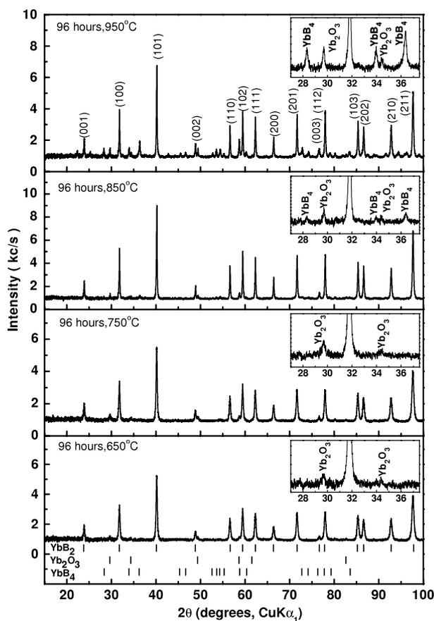
**Figure 1.** X-ray powder diffraction patterns of  $\text{YbB}_2$  samples heat treated at different temperatures for 96 h. Insets: the  $27\text{--}37.5^\circ$  region enlarged to identify major impurity phases;  $\text{YbB}_4$  and  $\text{Yb}_2\text{O}_3$ .
