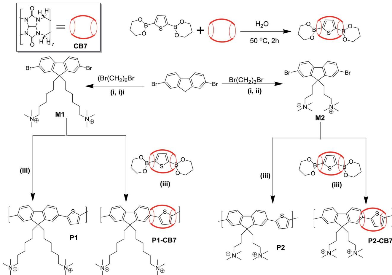
**Scheme 1** Synthetic schemes for poly[9,9-bis(6(*N,N,N*-trimethylamino)hexyl)fluorene-*co*-2,5-thienylene] (P1), poly[9,9-bis(3(*N,N,N*-trimethylamino)propyl)fluorene-*co*-2,5-thienylene] (P2) and their CB7-based polyrotaxane counter parts P1CB7 and P2CB7. Reaction conditions: (i) TBAB, 50% wt NaOH (aq), DMSO; (ii)  $\text{Me}_3\text{N}$ , THF, 25 °C, 24 h; (iii)  $\text{Pd}(\text{OAc})_2$ ,  $\text{K}_2\text{CO}_3$ ,  $\text{H}_2\text{O}$ , 80 °C, 48 h.
