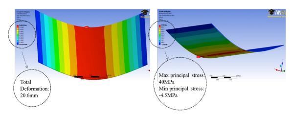
Fig. 8. The simple bending analysis results for the glass sheet under the load.
