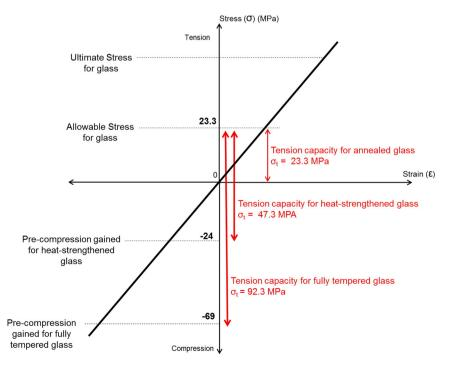
Fig. 3. The stress capacity of glass with different heat-treatments.
