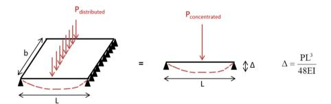
Fig. 7. Simple bending – deformation schema for the panel under linear load.
