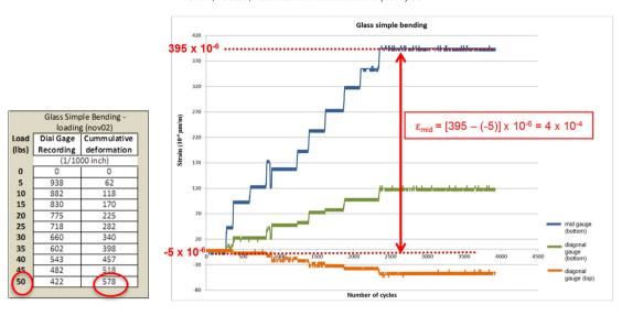
Fig. 9. The time history plot for the simple bending test.
