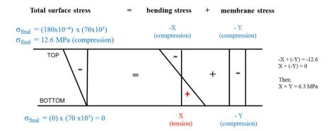
Fig. 11. Surface stresses on the deformed glass sheet.
