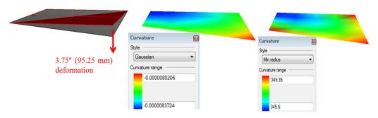
Fig. 12. Gaussian curvature and minimum radius analyses for the deformed sheet.
