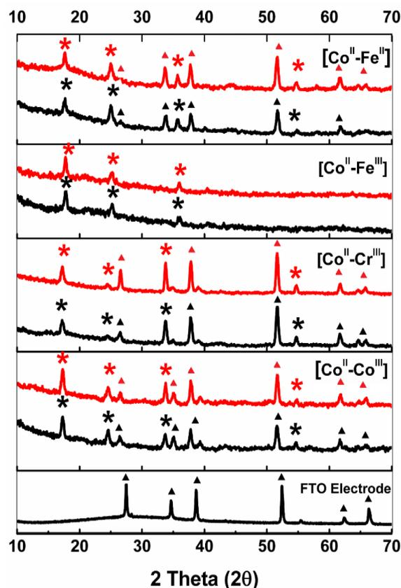
**Figure 4.** GI-XRD patterns of PB derivatives for pristine (black lines) and post catalytic (red lines). The peaks that belong to FTO electrode are marked with triangle (▲) and the peaks belong to Prussian Blue are marked with asterisk (\*).
