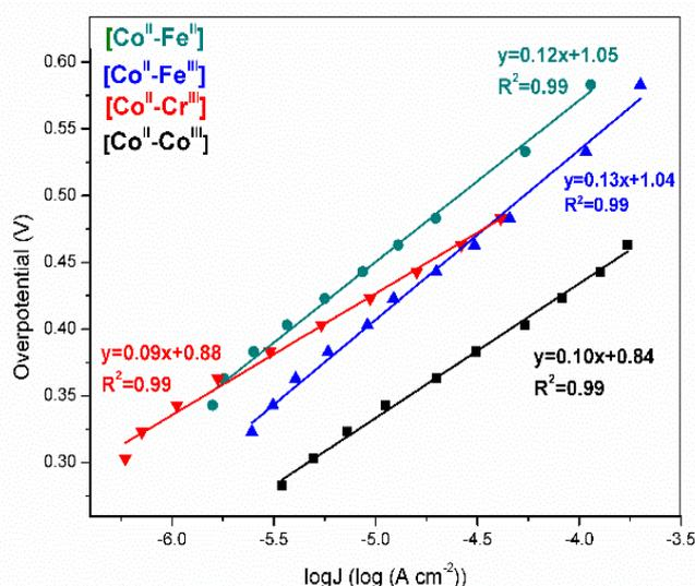
**Figure 2.** Tafel plots for PB derivatives from 1.1 to 1.4 V vs NHE recorded in a 50 mM KPi buffer at Ph 7.0.
