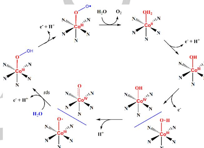
Figure 9. Proposed mechanism for water oxidation process for PBAs.
