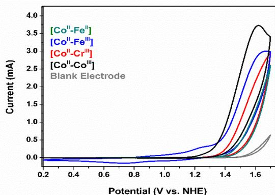
**Figure 1.** Cyclic Voltammograms of PB derivatives ( $[\text{Co}^{\text{II}}-\text{Co}^{\text{III}}]$  black,  $[\text{Co}^{\text{II}}-\text{Cr}^{\text{III}}]$  red,  $[\text{Co}^{\text{II}}-\text{Fe}^{\text{III}}]$  blue, and  $[\text{Co}^{\text{II}}-\text{Fe}^{\text{II}}]$  green lines) in 50 mM KPi electrolyte at pH 7 with  $50 \text{ mV sec}^{-1}$  sweep rate. The gray line indicates the electrochemical response of blank electrode.
