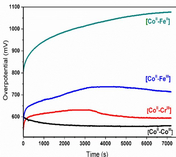
**Figure 3.** Chronopotentiometry measurement of PB derivatives at 1 mA cm<sup>-2</sup> in a 50 mM KPi buffer at pH 7.0
