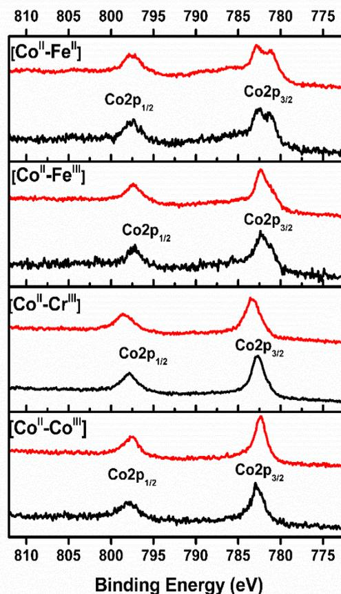
**Figure 5.** XPS of Co2p region for pristine (black lines) and post catalytic (red lines) of PB derivatives
