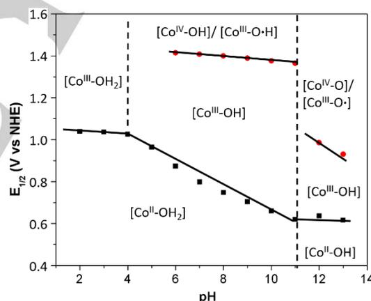
**Figure 7.** Pourbaix Diagram of  $[\text{Co}^{\text{II}}\text{-Co}^{\text{III}}]$  in KPI buffer at pHs from 2 to 13. Cyclic Voltammograms that are recorded at these pHs are shown in Figure (S10).
