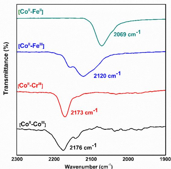
**Figure 6.** FTIR spectra of PB derivatives that shows cyanide stretches.
