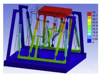
Fig. 4. FEM simulation of the system displacement.
