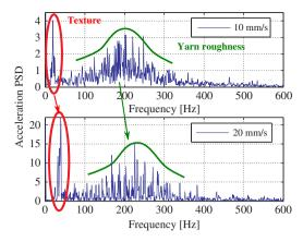
**Fig. 15.** An example of the acceleration PSD magnitude for the signals obtained from the accelerometer employing a textile sample.
