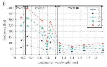
**Fig. 13.** Relationship between the frequency main peaks and the roughness width for different roughness samples: (a) subject 1 and (b) subject 2.
