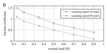
**Fig. 10.** (a) Friction coefficient between the fingertip and a steel surface sample with respect to the scanning velocity. (b) Friction coefficient between the fingertip and a steel surface sample with respect to the normal load for the extremes scanning speed employed during the measurements.
