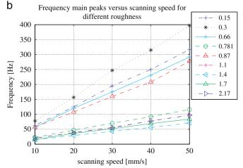
**Fig. 11.** Relationship between the frequency main peaks and the scanning speed for different roughness samples: (a) subject 1 and (b) subject 2.
