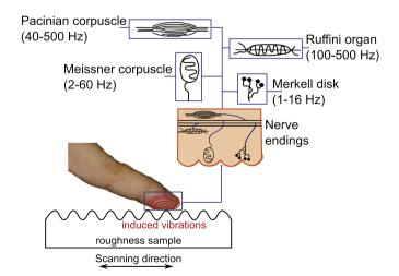
**Fig. 1.** Schematic representation of the contact between finger and object surface and scheme of the mechanoreceptors position into the skin. The scanning direction is along the line of the finger (from left to right, with respect to the figure).
