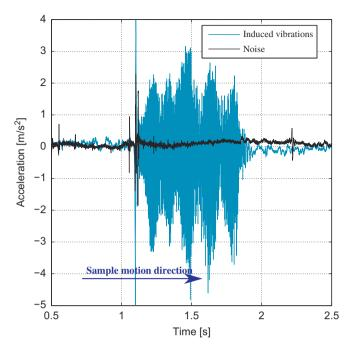
**Fig. 5.** An example of the comparison between the acquired acceleration signal of the vibrations induced by the fingertip/surface scanning and the parasite noise from the set-up functioning. (For interpretation of the references to color in this figure, the reader is referred to the web version of this article.)
